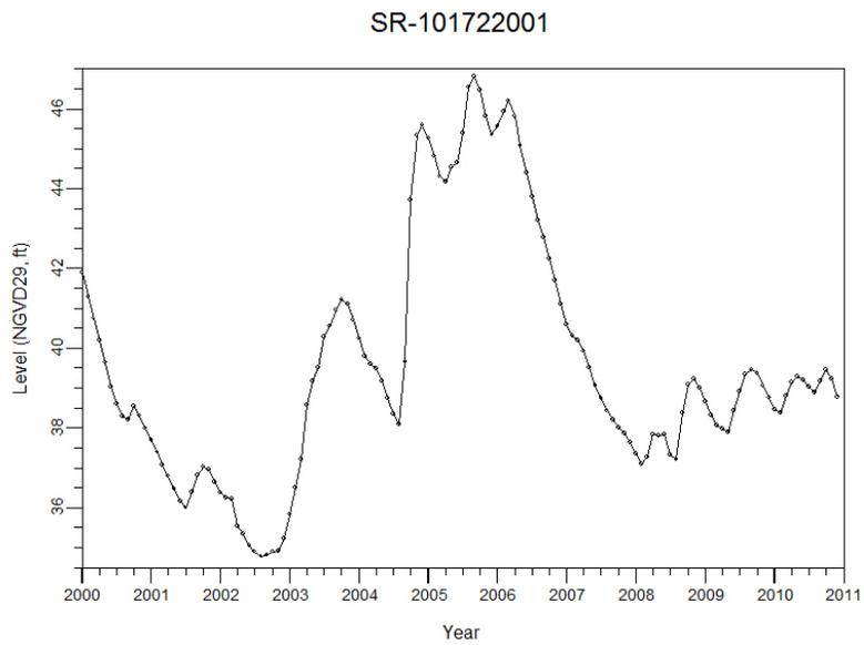
**Figure 90. Hydrograph of Well SR-101722001 (Site 67; Cluster 8).**
