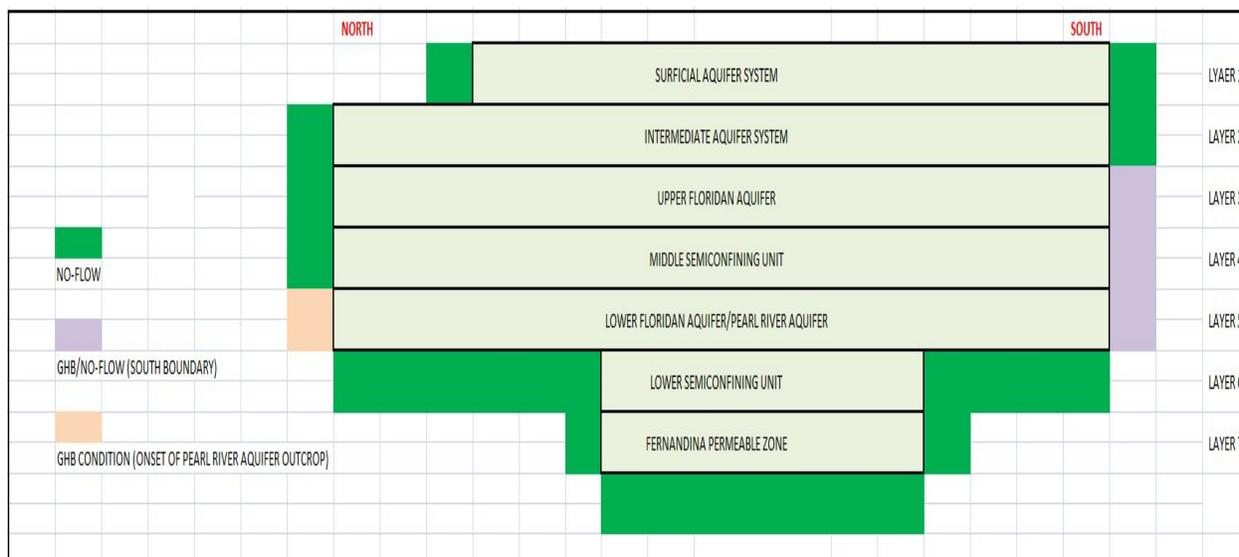
**Figure 6. Generalized Model Layer and Lateral Boundary Condition Diagram (NORTH-SOUTH).**
