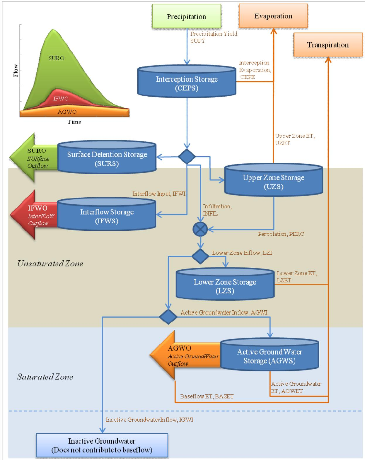
Figure 22. Illustration of water storage and movement in the HSPF model pervious land element (PERLND).
