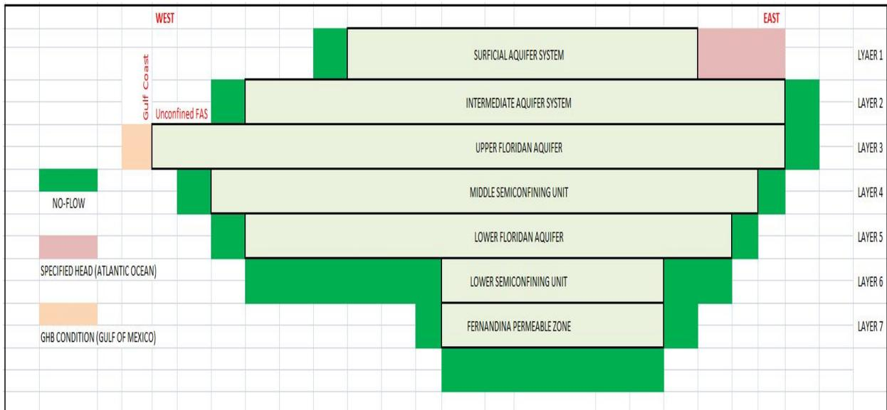
Figure 5. Generalized Model Layer and Lateral Boundary Condition Diagram (WEST-EAST).
