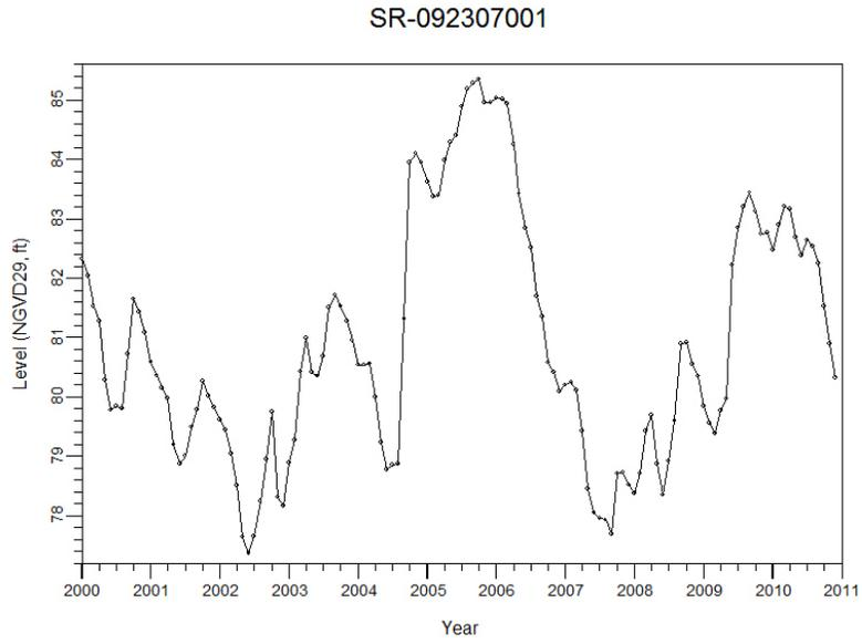
**Figure 89. Hydrograph of Well SR-092307001 (Site 66; Cluster 7).**
