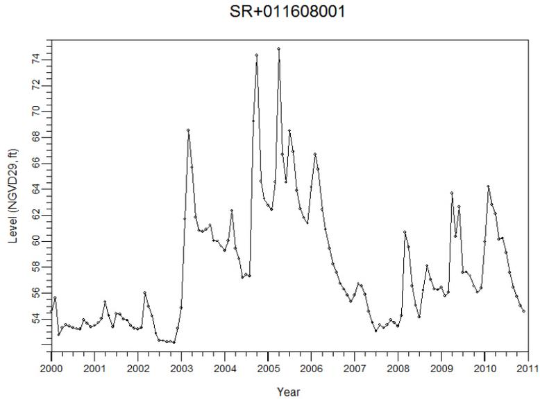
**Figure 51. Hydrograph of Well SR+011608001 (Site 27; Cluster 5).**
