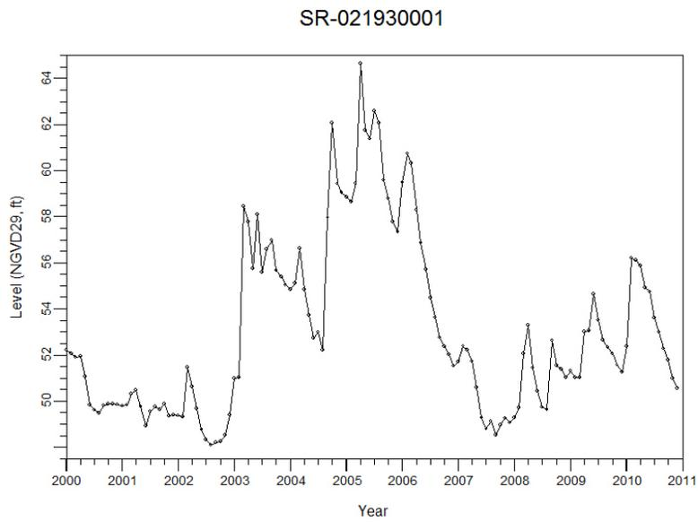
**Figure 72. Hydrograph of Well SR-021930001 (Site 48; Cluster 6)**
