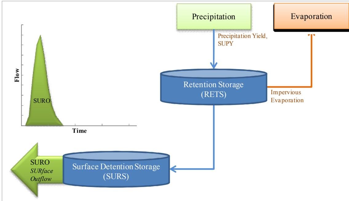
Figure 23. Illustration of water storage and movement in the HSPF model impervious land element (IMPLND).
