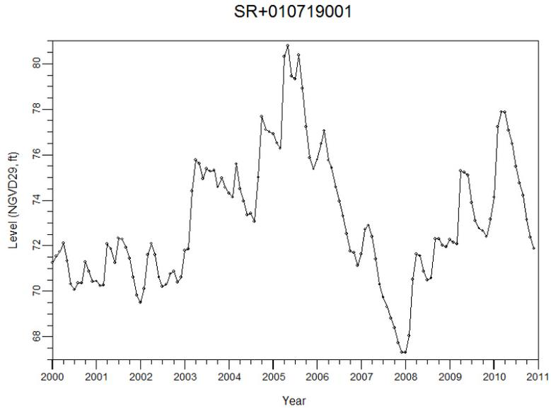
**Figure 67. Hydrograph of Well SR+010719001 (Site 43; Cluster 6).**
