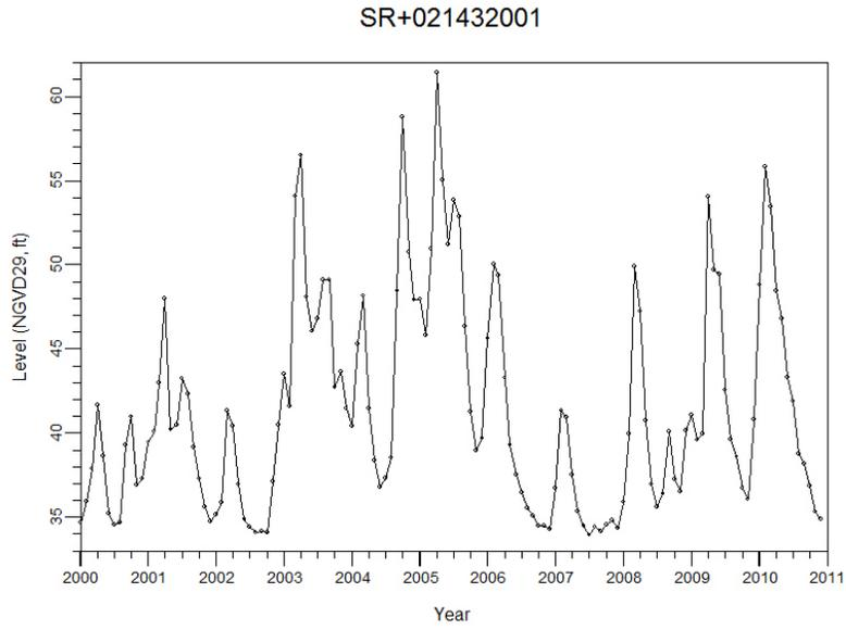
**Figure 53. Hydrograph of Well SR+021432001 (Site 29; Cluster 5).**
