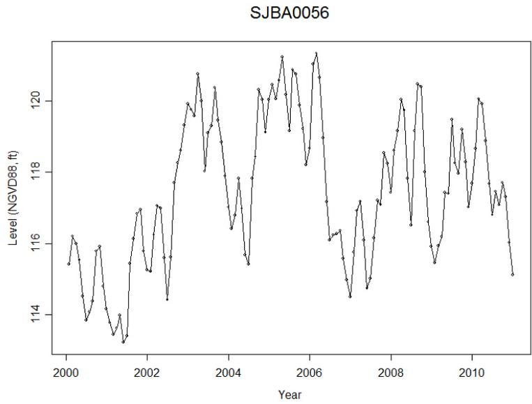
**Figure 96. Hydrograph of Well SJBA0056 (Site 4).**
