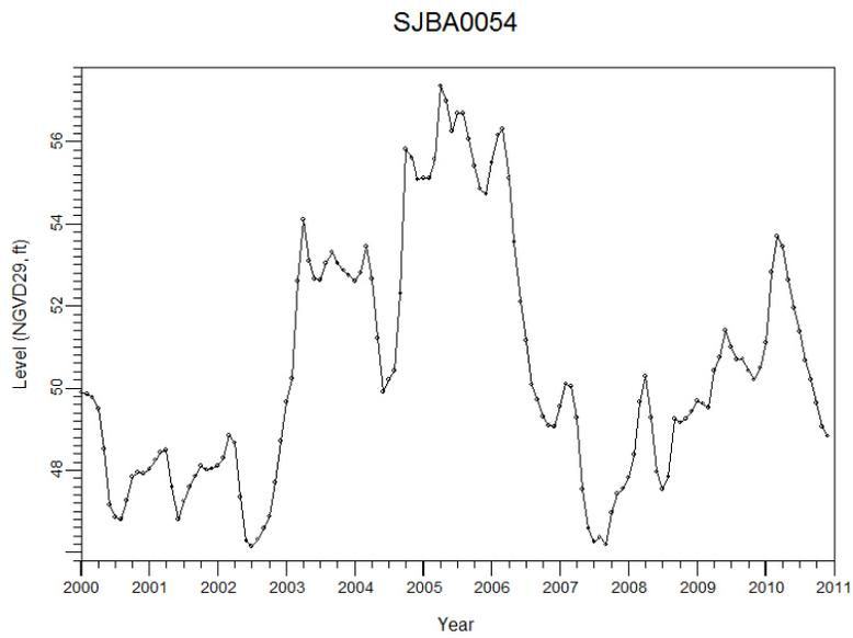
**Figure 62. Hydrograph of Well SJBA0054 (Site 38; Cluster 6).**
