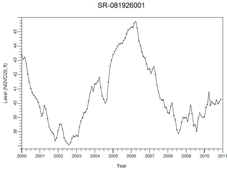
**Figure 92. Hydrograph of Well SR-081926001 (Site 69; Cluster 8).**
