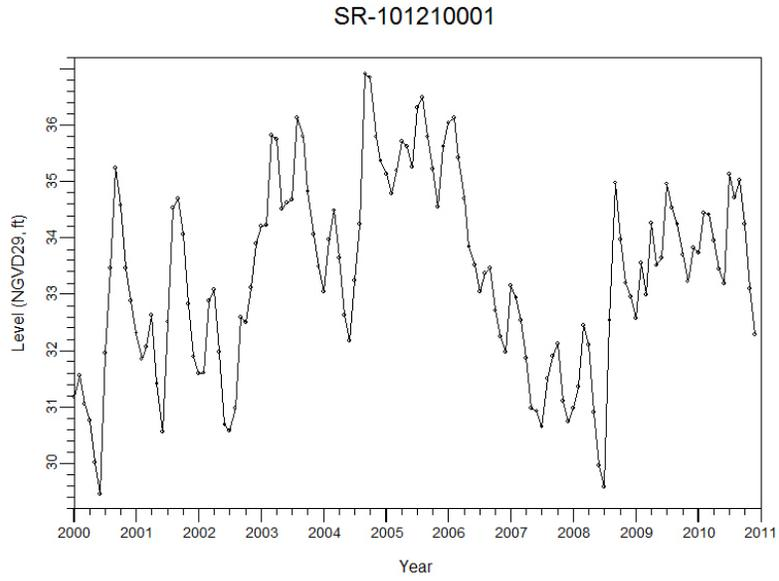
**Figure 33. Hydrograph of Well SR-101210001(Site 9; Cluster 2).**
