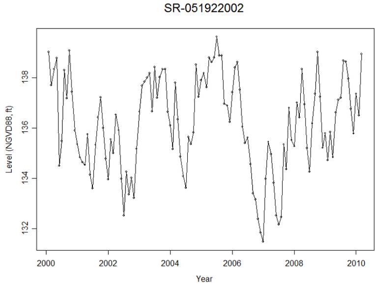
**Figure 103. Hydrograph of Well SR-051922002 (Site 11).**
