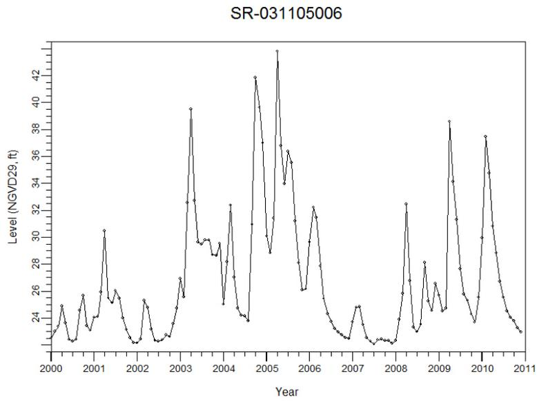
**Figure 54. Hydrograph of Well SR-031105006 (Site 30; Cluster 5).**
