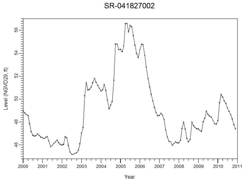
**Figure 74. Hydrograph of Well SR-041827002 (Site 50; Cluster 6).**
