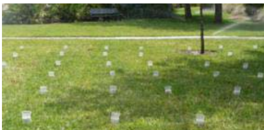
Figure 28. A catch-can test used to determine distribution uniformity.
