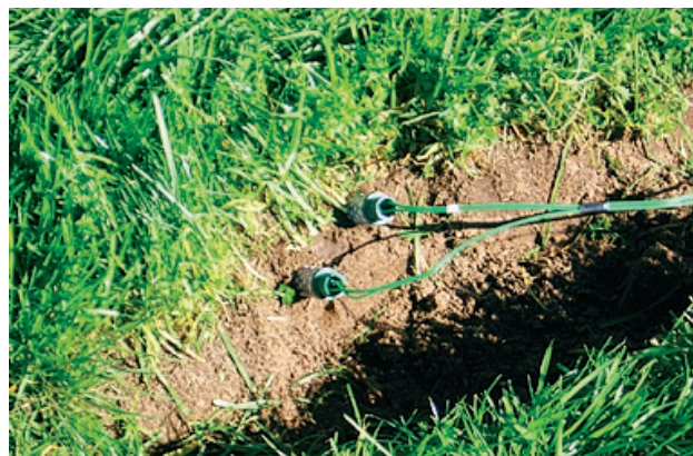
Figure 21. SMS node probes installed in turf root zone
