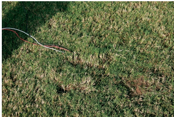
Figure 19. Soil and turf grass plug replaced, covering SMS probe prior to burying wire
