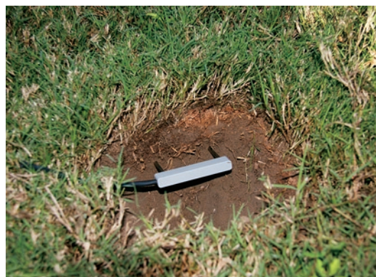
Figure 22. SMS rod probes partially inserted into the turf grass root zone of undisturbed soil
