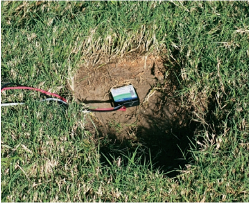
Figure 17. SMS probe installed within root zone
