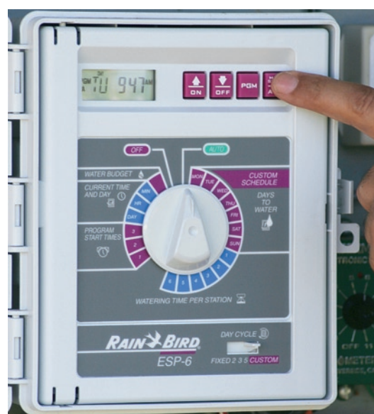
Figure 40. Manual start of the irrigation timer to saturate area around SMS for calibration
