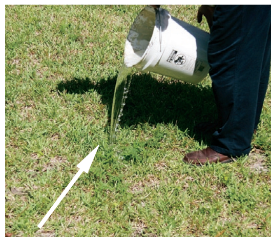
Figure 39. Establishing the controller set point—bucket method (arrow points to sensor location)
