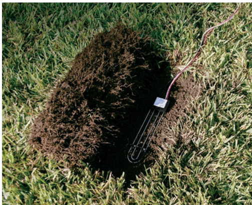
Figure 12. SMS installed in root zone by rolling back the sod
