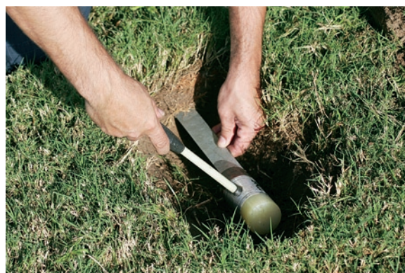
Figure 16. Root cutting procedure preparing soil for SMS installation
