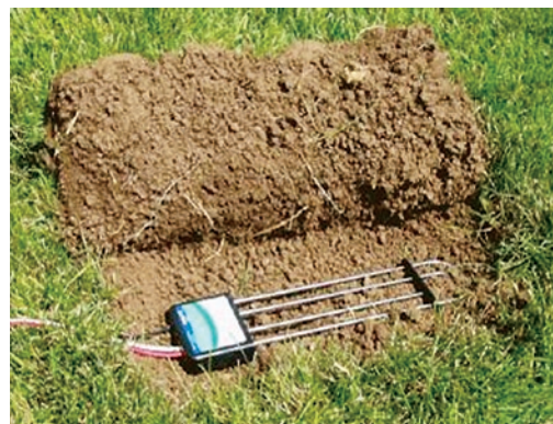
Figure 7. Probe with exposed wave guides
