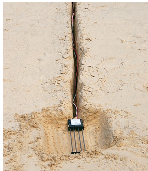
Figure 9. Installation of flat probe SMS in new landscape (bare soil)
