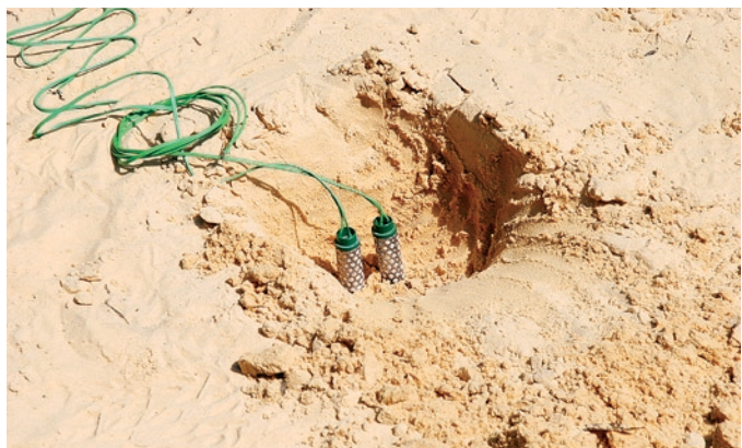
Figure 20. SMS node probes in a new landscape installation
