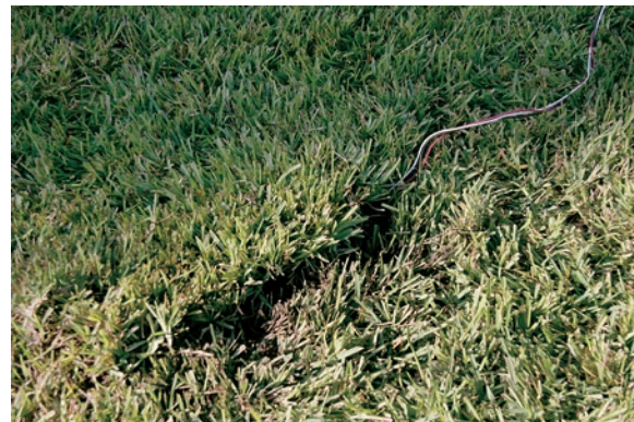
Figure 13. Turf grass rolled back over sensor
