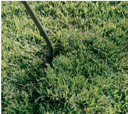
Figure 10. Cutting a square of turf grass large enough to cover entire probe
