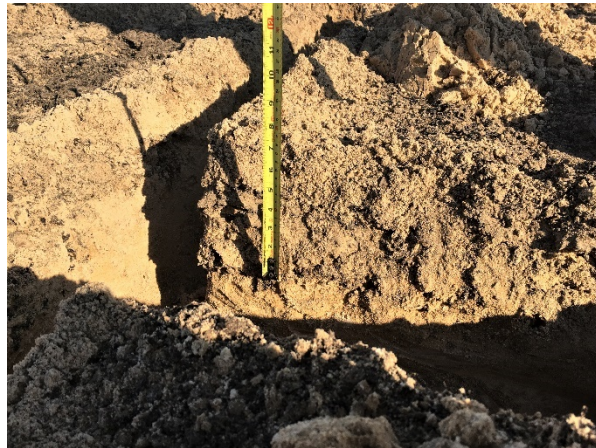
Figure 12. Check for a general 6-inch incorporation depth, 4-inch minimum in small areas. Credit: UF/PREC.
