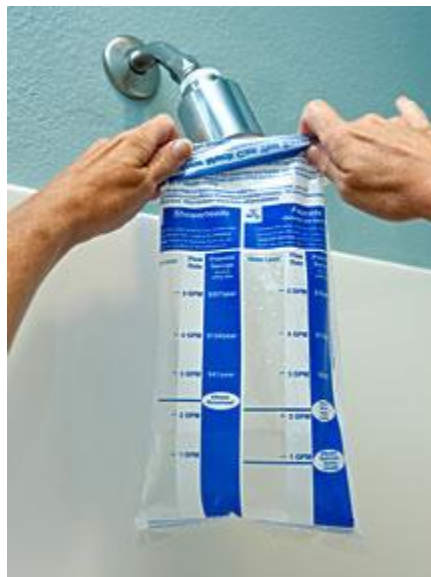
Testing a showerhead using a flow bag
