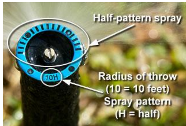
Pop-up sprinkler head indicating spray pattern and distance of throw
