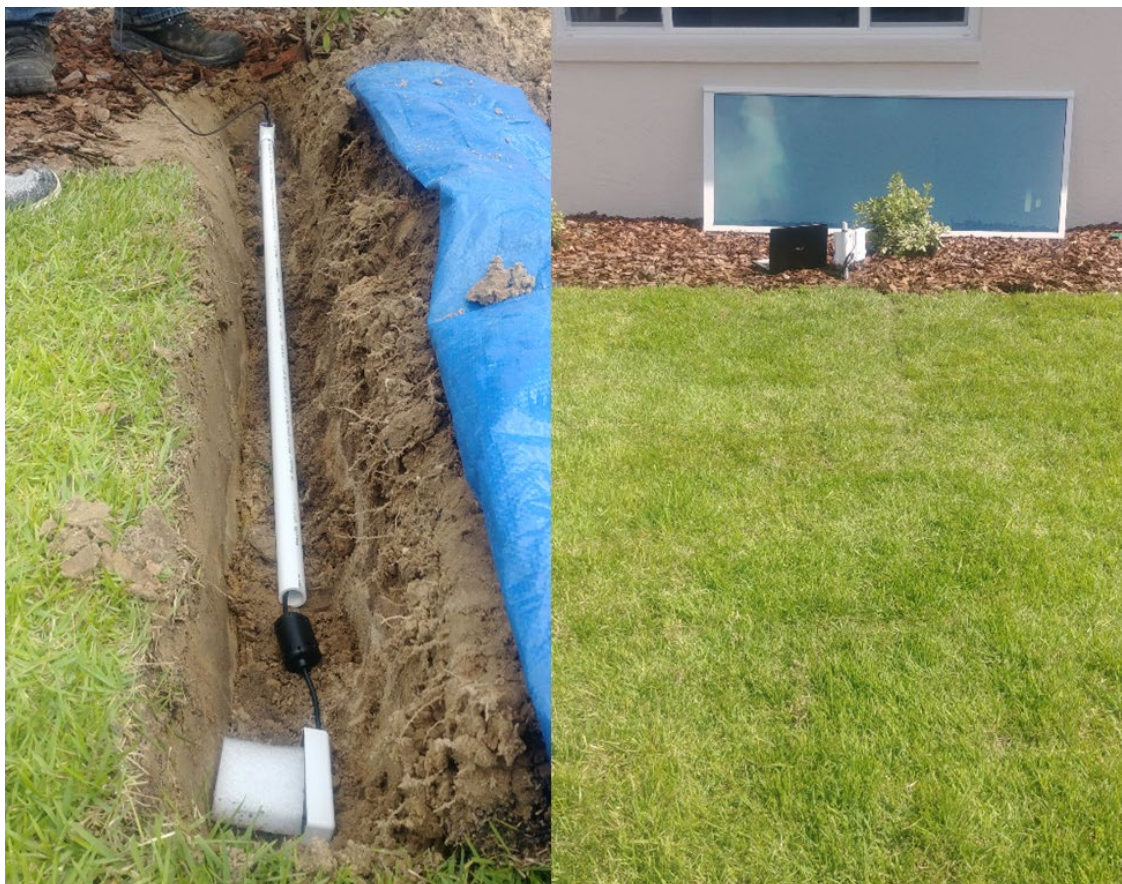
Figure 2-7. Installation of a Teros-12 soil moisture sensor with the cable housed in pvc pipe (left) and after installation connected to an Em50 data logger (right).
