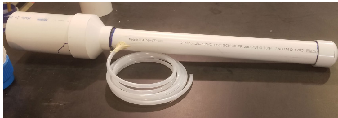
Figure 2-9. Fully constructed lysimeter showing the collection chamber as well as the leachate reservoir and the positioning of the sample collection tube.
