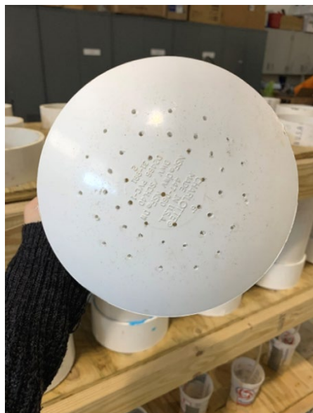
Figure 2-16. Small holes drilled into a 15 cm (6 in) PVC cap to distribute irrigation evenly over the column and minimize disturbance.
