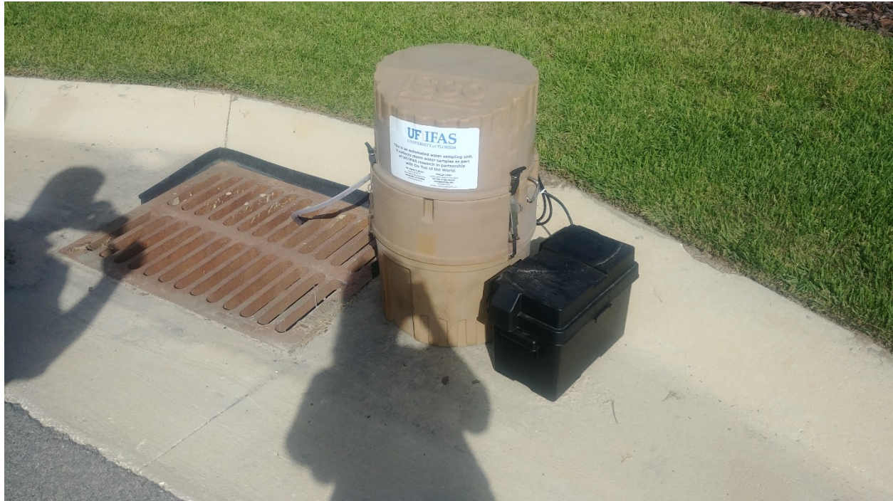
Figure 2-6. ISCO 3712 autosampler and battery positioned next to a storm drain that is equipped with a Visqueen sheet, plastic barrier to direct runoff into the weir box, and collection tube, prepared for sample collection.
