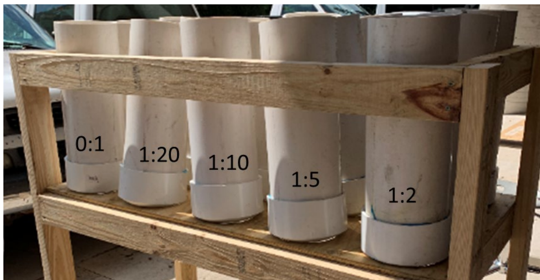
Figure 2-12. Soil columns arranged five across and three deep on rack with amendment/soil ratios labeled on the columns.
