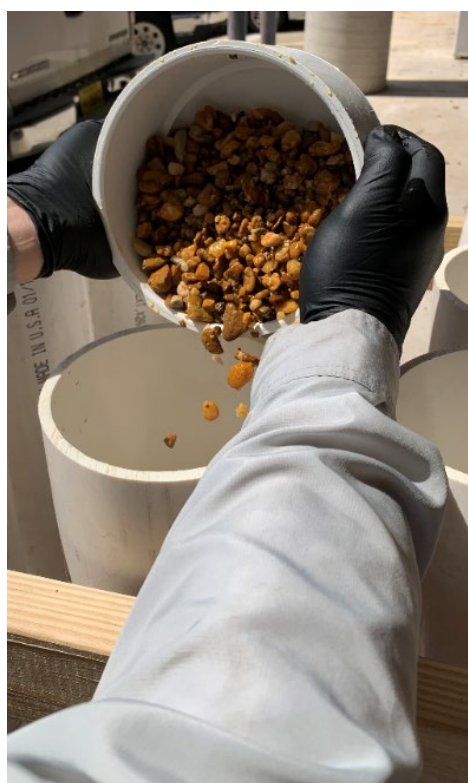
Figure 2-13. Adding 2 in. (5 cm) of washed pea gravel to the bottom of each column to limit soil washout.
