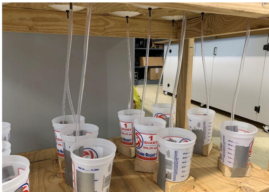
Figure 2-15. Coupler attached to a collection tube which is taped to the inside of a catch can.
