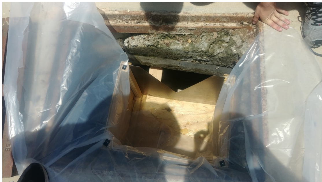
Figure 2-3. Weir box with 60° weir plate and Visqueen covering the sides to direct all water into and through the weir box for flow measurement.
