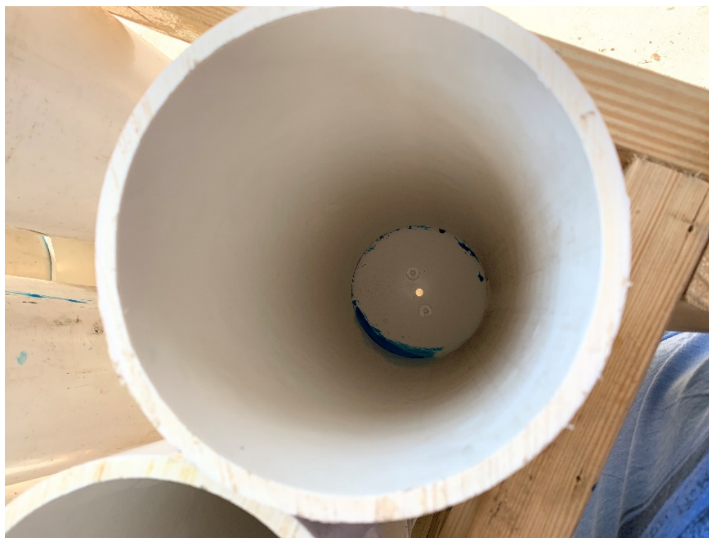
Figure 2-14. Columns showing the 3/8 in. (0.95 cm) hole drilled into the bottom to allow for drainage.
