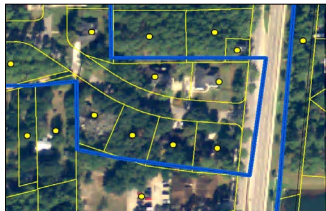
Figure 5. Parcel centroids (yellow points) used in summarizing parcels (yellow polygons) to utility service area boundaries (blue polygons)
