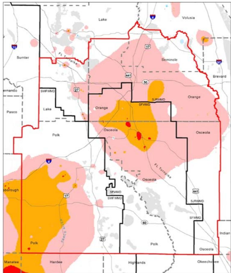
Changes of Simulated Mean Water Levels in Model Layer 3 (Upper Floridan Aquifer) between the 2014 Reference Condition and 2040 Withdrawals Condition
